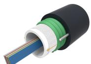
Fiber OSP cable, Steel Armored, Gel-Filled Central Tube Ribbon, 192 fiber, Multimode OM4, bend insensitive, Feet jacket marking, Black jacket color
