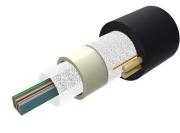
Fiber OSP Cable, Non-Armored, All-Dielectric, Arid-Core, Dry Central Tube Ribbon, 12 fibers, Singlemode G.652.D and G.657.A1, Gel-free, Feet jacket marking, Black jacket color
