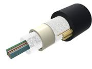
Fiber OSP Cable, Non-Armored, All-Dielectric, Arid-Core, 216 fiber, Dry Central Tube Ribbon, Singlemode G.652.D and G.657.A1, Gel-free, Feet jacket marking, Black jacket color
