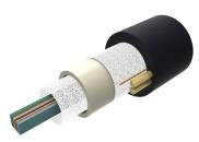
Fiber OSP Cable, Non-Armored, All-Dielectric, Arid-Core, 360 fiber, Dry Central Tube Ribbon, Singlemode G.652.D and G.657.Al, Gel-free, Feet jacket marking, Black jacket color
