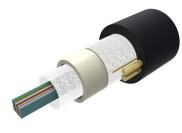
Fiber OSP Cable, Non-Armored, All-Dielectric, Arid-Core, Dry Central Tube Ribbon, 12 fibers, Multimode OM3 bend insensitive, Gel-free, Feet jacket marking, Black jacket color
