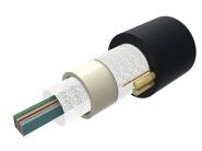
Fiber OSP Cable, Non-Armored, All-Dielectric, Arid-Core, Dry Central Tube Ribbon, Multimode OM3 bend insensitive, Gel-free, Feet jacket marking, Black jacket color
