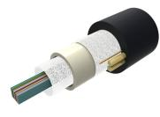
Fiber OSP Cable, Non-Armored, All-Dielectric, Arid-Core, 48 fibers, Dry Central Tube Ribbon, Multimode OM4 bend insensitive, Gel-free, Feet jacket marking, Black jacket color
