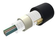
Fiber OSP Cable, Non-Armored, All-Dielectric, Arid-Core, 60 fibers, Dry Central Tube Ribbon, Multimode OM4 bend insensitive, Gel-free, Feet jacket marking, Black jacket color
