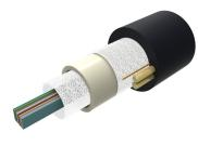
Fiber OSP Cable, Non-Armored, All-Dielectric, Arid-Core, 72 fiber, Dry Central Tube Ribbon, Multimode OM4 bend insensitive, Gel-free, Feet jacket marking, Black jacket color
