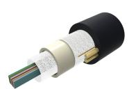
Fiber OSP Cable, Non-Armored, All-Dielectric, 144 fiber, Arid-Core, Dry Central Tube Ribbon, Multimode OM4 bend insensitive, Gel-free, Feet jacket marking, Black jacket color
