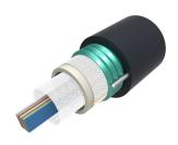
Fiber OSP cable, Steel Armored, Arid-Core, Dry Central Tube Ribbon, 36 fiber, Multimode OM4, bend insensitive, Feet jacket marking, Black jacket color
