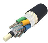
Fiber OSP Cable, Non-Armored, All-Dielectric, 864 fiber, Gel-Filled Loose Tube Ribbon, Multimode OM4 bend insensitive, Feet jacket marking, Black jacket color
