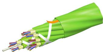
Fiber indoor cable, LazrSPEED® Plenum MPO Trunk, 144 fiber multi-unit with 12 fiber subunits, Multimode OM5, Gel-free, Feet jacket marking, Lime green jacket color
