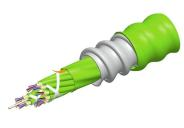
Fiber indoor cable, LazrSPEED® Riser Distribution, interlocking aluminum armored, Multimode OM5, 36 fiber multi-unit with 12 fiber subunits, Limegreen jacket color, Feet cable marking
