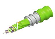
Fiber indoor cable, LazrSPEED® Plenum MPO Trunk, interlocking aluminum armored with plenum jacket, Multimode OM5, 36 fiber multiunit with 12 fiber subunits, Lime-green jacket color, Feet cable marking
