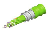
Fiber indoor cable, LazrSPEED® Riser/LSZH rated, MPO Trunk, interlocking aluminum armored, Multimode OM5, 12 fiber, Feet jacket marking, Lime-green jacket color
