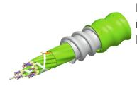
Fiber indoor cable, LazrSPEED® Riser/LSZH rated MPO Trunk, interlocking aluminum armored, 72 fiber multi-unit with 12 fiber subunits, Feet jacket marking, Lime-green jacket color
