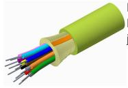
Fiber indoor cable, LazrSPEED® Low Smoke Zero Halogen Riser Distribution Cable, 24 fiber single-unit, Gel-free, Multimode OM5, Feet jacket marking, Lime green jacket color, Dca flame rating
