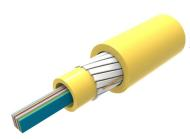
Fiber Indoor Cable, Plenum All-Dielectric Central Tube Ribbon, 96-fiber, Singlemode G.652.D and G.657.Al, Feet jacket marking, Yellow jacket color
