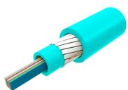
Fiber Indoor Cable, Multimode OM3 bend insensitive, 12 fibers, Plenum, All-Dielectric Central Tube Ribbon, Gel-free, Feet jacket marking, Aqua jacket color
