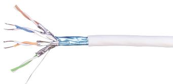
3296A-B Category 6A F/FTP Cable, low smoke zero halogen, white jacket, 4 pair count, 1640 ft (500 m) length, reel
