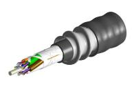
Fiber indoor/outdoor cable, LazrSPEED®, Plenum Rated, Gel-Free, Multimode OM5, 6 fiber, Stranded Loose Tube with Aluminum Interlocking Armor containing a Plenum Rated Outer Jacket, Feet jacket marking, Black jacket color
