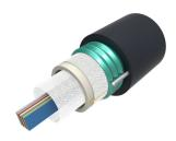
Fiber OSP cable, Steel Armored, Arid-Core, Dry Central Tube Ribbon, 720 fiber, Singlemode G.652.D and G.657.A1, Feet jacket marking, Black jacket color
