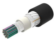
Fiber indoor/outdoor cable, All-Dielectric, LSZH Riser-Rated, Gel-Free, Central Tube Rollable Ribbon, 288 fiber, Singlemode G.652.D and G.657. Al, Feet jacket marking, Black jacket color, Cca flame rating
