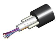
Fiber Indoor/Outdoor cable, Single Jacket Gel-Filled All-Dielectric, 48 fibers, Riser Rated Central Tube, Singlemode G.657.A2/B2, Feet jacket marking, Black jacket color
