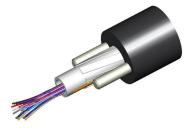
Fiber Indoor/Outdoor cable, Single Jacket Gel-Filled All-Dielectric, 48 fibers, Riser Rated Central Tube, Singlemode G.657.A2/B2, Feet jacket marking, Black jacket color
