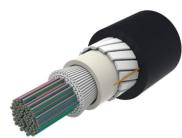
Fiber indoor/outdoor cable, LSZH Riser Rollable Ribbon, 864 fiber, Singlemode G.652.D and G.657.A1, Gel-free, Feet jacket marking, Black jacket color, Cca flame rating
