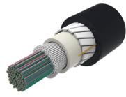
Fiber indoor/outdoor cable, LSZH Riser Rollable Ribbon, 864 fiber, Singlemode G.652.D and G.657.A1, Gel-free, Feet jacket marking, Black jacket color, Cca flame rating
