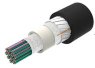
Fiber indoor/outdoor cable, All-Dielectric, LSZH Riser-Rated, Gel-Free, Central Tube Rollable Ribbon, 192 fiber, Singlemode G.657.A2/B2, Feet jacket marking, Black jacket color, Cca flame rating
