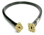
FlexTwist® Flexible Twist for WR90, 8.2–12.4 GHz, with interface types PDR100 and PBR100, 600 mm
