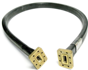
FlexTwist® Flexible Twist for WR90, 10.7–11.7 GHz, with interface types PBR100 and PBR100, 600 mm
