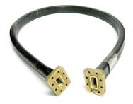
FlexTwist® Flexible Twist for WR112, 7.125–8.5 GHz, with interface types CPR112G and CPR112G, 600 mm
