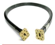
FlexTwist® Flexible Twist for WR112, 7.05–10.0 GHz, with interface types CPR112G and CMR112, 1200 mm
