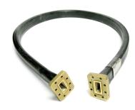
FlexTwist® Flexible Twist for WR112, 7.05–10.0 GHz, with interface types CPR112G and PDR84, 900 mm
