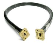
FlexTwist® Flexible Twist for WR112, 7.125–8.5 GHz, with interface types PDR84 and PBR84, 900 mm
