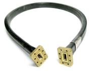
FlexTwist® Flexible Twist for WR112, 7.05–10.0 GHz, with interface types PBR84 and UDR84, 900 mm
