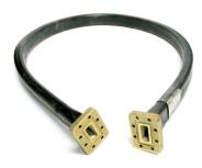
FlexTwist® Flexible Twist for WR112, 7.05–10.0 GHz, with interface types PBR84 and UBR84, 600 mm
