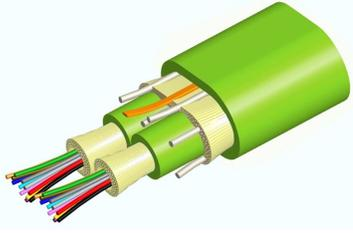
Fiber indoor cable, LazrSPEED®, Low Smoke Zero Halogen Riser MPO Trunk, 24 fiber with 12 fiber subunits, Gel-free, Multimode OM5, Feet jacket marking, Dca flame rating
