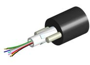
Fiber drop cable, LazrSPEED® Single Jacket All-Dielectric Arid Core, 12-fiber, Multimode OM3, Gel-filled, Feet jacket marking, Black jacket color
