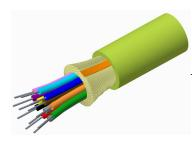
Fiber indoor cable, LazrSPEED® Low Smoke Zero Halogen Riser Distribution Cable, 24 fiber single-unit, Gel-free, Multimode OM5, Feet jacket marking, Lime green jacket color, B2ca flame rating
