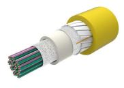
Fiber indoor cable, All-Dielectric, LSZH/Riser-Rated, Gel-Free, Central Tube Rollable Ribbon, 576 fiber, Singlemode G.657.A2, Feet jacket marking, Yellow jacket color, Cca flame rating
