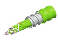
Fiber indoor cable, LazrSPEED® Plenum MPO Trunk, interlocking aluminum armored with plenum jacket, Multimode OM5, 72 fiber multiunit with 12 fiber subunits, Lime-green jacket color, Feet cable marking
