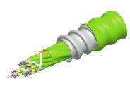
Fiber indoor cable, LazrSPEED® Plenum MPO Trunk, interlocking aluminum armored with plenum jacket, Multimode OM5, 144 fiber multiunit with 12 fiber subunits, Lime-green jacket color, Feet cable marking
