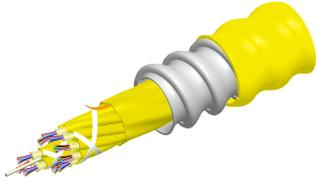
Fiber indoor cable, Plenum MPO Trunk, interlocking aluminum armored with plenum jacket, 36 fiber multi-unit with 12 fiber subunits, Gel-free, Singlemode G.657.A2, Feet jacket marking, Yellow jacket color
