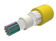
Fiber indoor cable, All-Dielectric, LSZH/Riser-Rated, Gel-Free, Central Tube Rollable Ribbon, 192 fiber, Singlemode G.657.A2/B2, Feet jacket marking, Yellow jacket color, Cca flame rating
