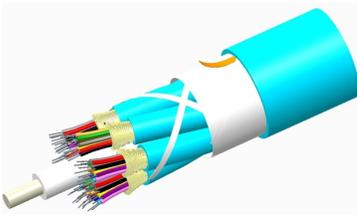
Fiber indoor cable, TeraSPEED® Low Smoke Zero Halogen Riser Distribution, 72 fiber multi-unit with 12 fiber subunits, Gel-free, Singlemode + Multimode OM3, Feet jacket marking, Aqua jacket color
