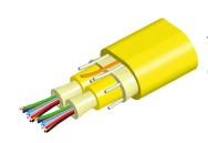
Fiber indoor cable, TeraSPEED® Low Smoke Zero Halogen Riser MPO Trunk, 24 fiber with 12 fiber subunits, Gel-free, Singlemode G.652.D and G. 657.A1, Feet jacket marking, Yellow jacket color, Dca flame rating
