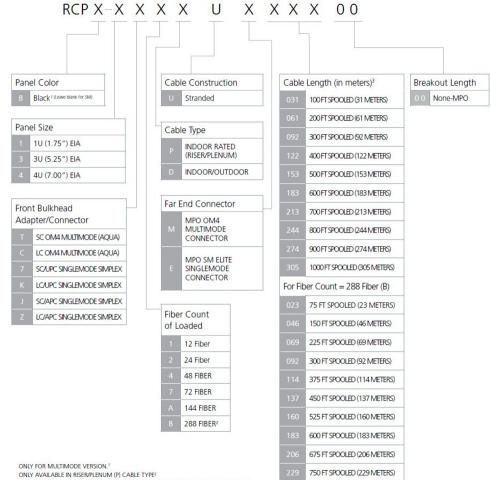
RAPID PANEL IS DESIGNED AND QUALIFIED FOR UP TO 1000' (305 METERS) OF CABLE.<sup>3</sup>
