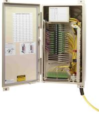
Enhanced Mini FDH, 72F loaded pole/wall mounted cabinet, SC/APC, PNP splitter capable, Loose Tube pigtailed splice cabinet capable of receiving 24F and distributing 72F via provided splice trays
