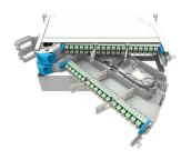
MFPS Fiber Optic panel, 2RU, 72 fibers/RU, splice/patch, SMOUV/front patch cords orientation to the left, 144 LC/APC, grade C
